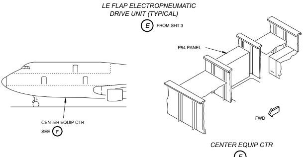
Lift Augmenting - Component Location Figure 102 (Sheet 4)
